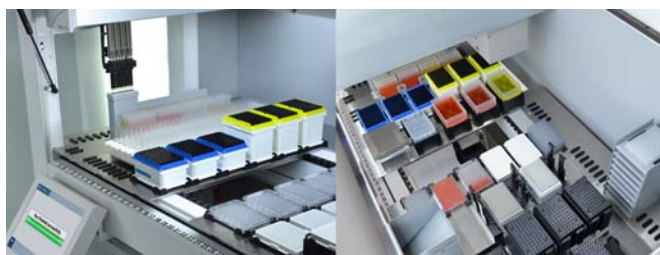
Figure 2: Dynamic Deck with six ANSI/SLAS positions in the depth, equipped with six boxes for disposable tips for the Flexible Channel Arm on the left. Blue colour code for 200µl and yellow colour code for 1000µl disposable tips. Top view of the Dynamic Deck on the right showing nested disposable tips, positions for troughs, active carrier for the MCA 384 and a hotel in the back.
